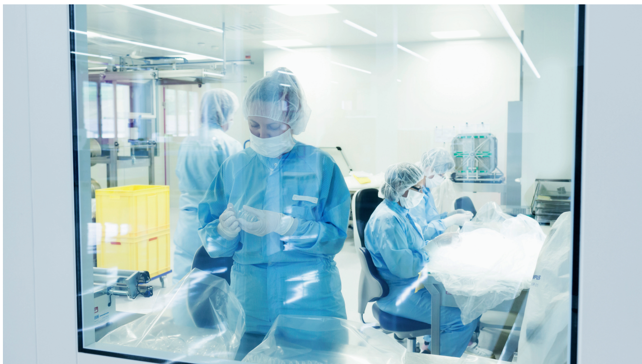
Production in a cleanroom: in Stein am Rhein in Switzerland, Trelleborg can produce and pack in cleanrooms of class 7 and 8 according to ISO 14644-1 (class 10,000 and class 100,000 according to US FED 209D) © Trelleborg
